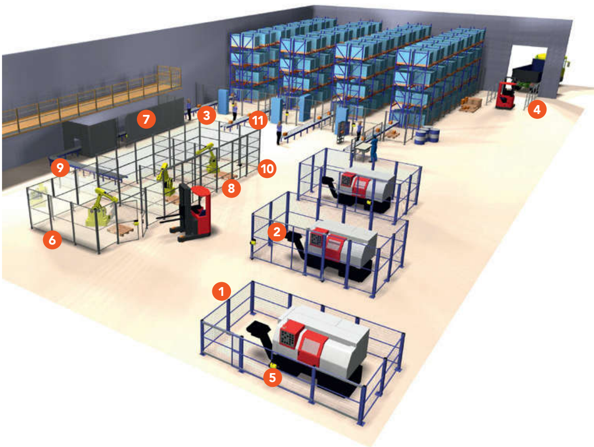
6 Roller on wheels – up to approximately 2.5m high. Equipped with ST30 mesh panels.
