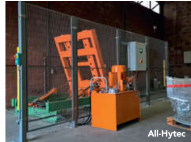
1 Strong Fix Our strongest machine guard that can withstand an impact of 2,500 joules.
